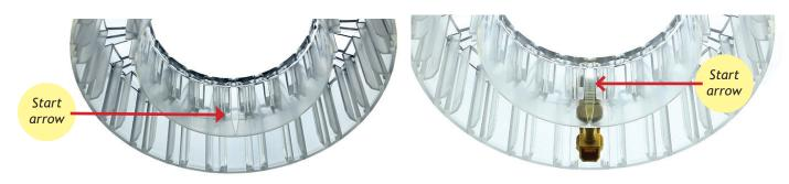
Looking straight down on the drum, put the next tag in the sequence to the left of the first tag. For single tags, this will be the next tag number in the sequence.
