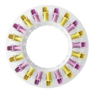
Push every tag firmly into place so the bend in the tag is flush with the back of the drum cartridge. Check the back of the drum cartridge to make sure no tag is pushed too far - tags that are poking out the back will cause the applicator to jam!
