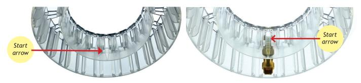
Looking straight down on the drum, put the next tag in the sequence to the left of the first tag. For paired tags this will be the matching tag number to the first tag.
